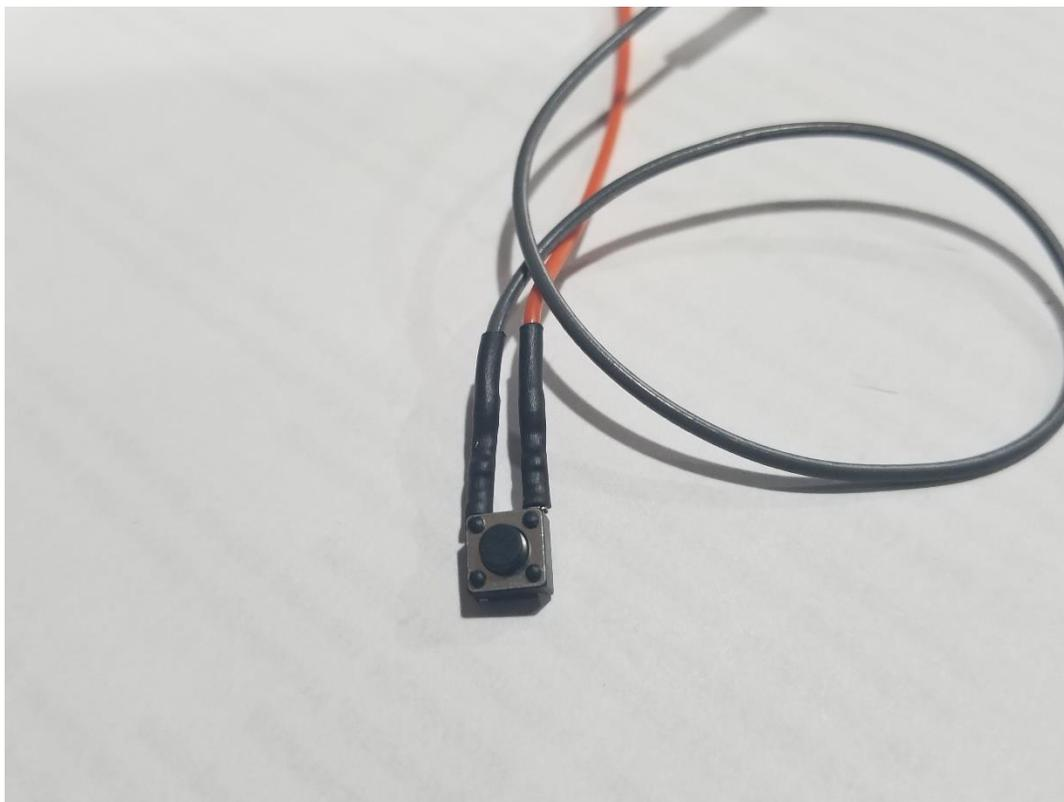
*(Image 13 - Momentary Switch Connected to Jumpers)*
