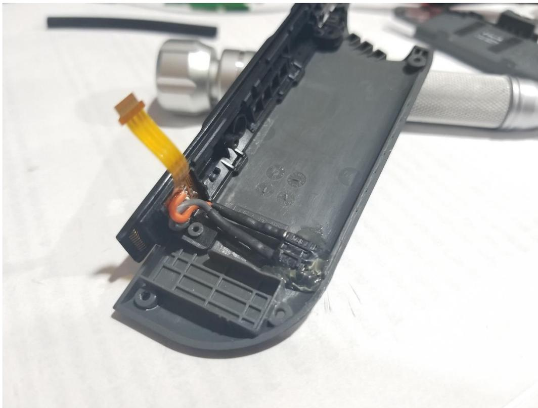
*(Image 24 - JoyCon Slide Connector Board Connected to the Momentary Switch and JoyCon Back)*
