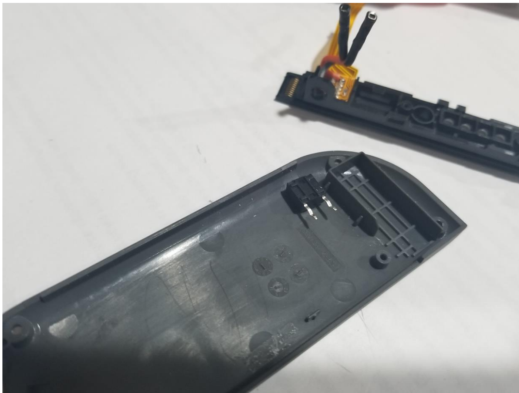
(Image 16 - Using Momentary Switch to Find the Drill Location)
