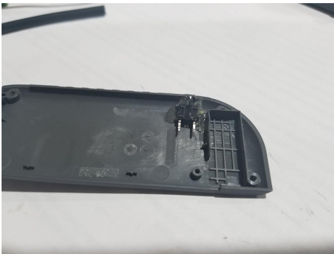
(Image 18 - Momentary Switch Secured with Hot Glue)
