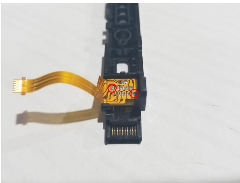
(Image 21 - Solder Posts for Pins 1 & 10 Circled in Red)
