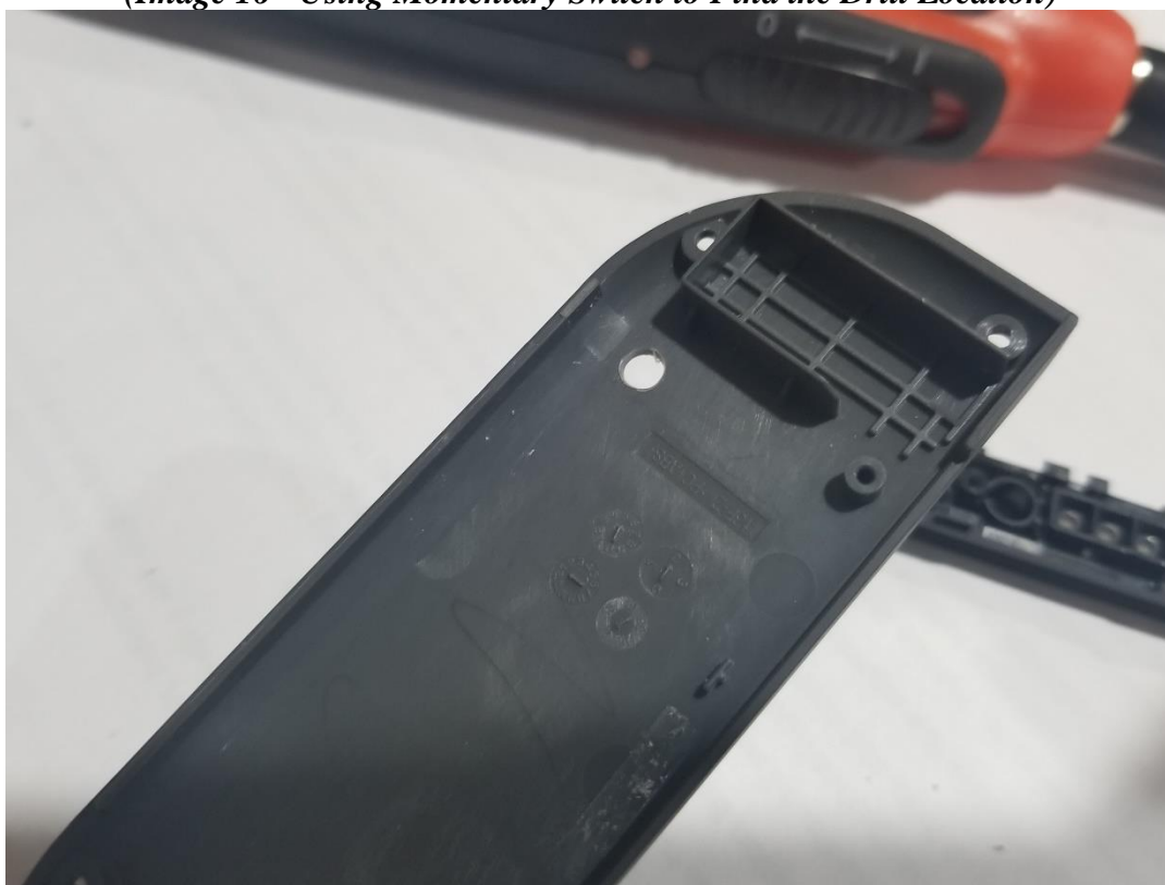
(Image 17 - Drilled Hole on the Back of the JoyCon Controller (A Little too Far to the Left))
