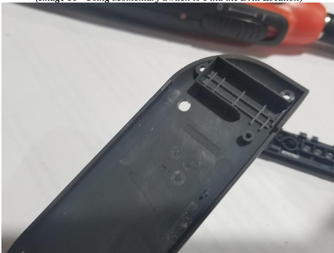
*(Image 17 - Drilled Hole on the Back of the JoyCon Controller (A Little too Far to the Left))*
