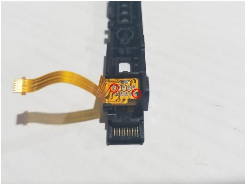
*(Image 21 - Solder Posts for Pins 1 & 10 Circled in Red)*
